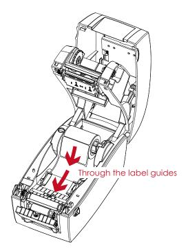
3. Pull the label liner through the platen and the steel of the label dispenser.
