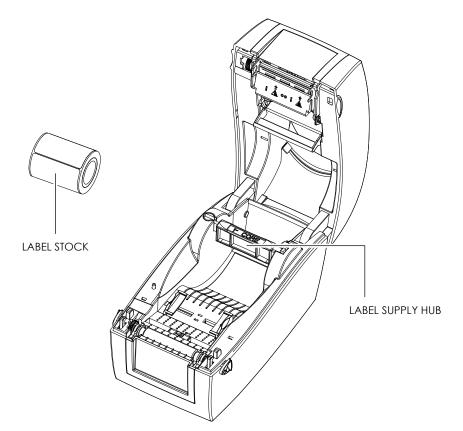
1. Unlock the release catch to lift the label supply hub.
