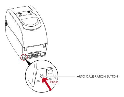
Calibration button can be used to find correct printing position or eliminate the "Media Error" problem.
