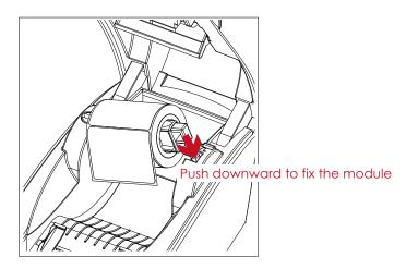
4. A new label supply module is completed.
