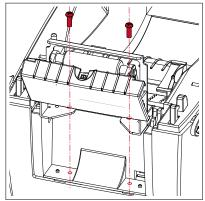
3. Place the platen back to the printer and lock the clips.
