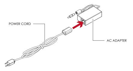
Connect the jack of the power adapter to the printer and connect the plug of the power adapter to the socket of the wall.
